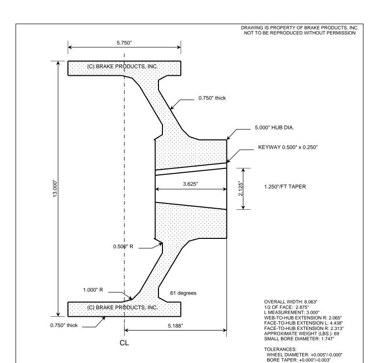
SIGNATURE: APPROVED BY: DATE: 0 Н F В S Т D WHEEL DIAMETER FACE WIDTH HUB OFFSET HUB LENGTH BORE DIAMETER BORE TAPER IN/FT KEYWAY WIDTH KEYWAY DEPTH
